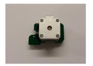
Turn the block over, and fasten the motor with four M3x12mm cap head screws. Don't fully tighten these; the motor, spacer and block need to be able to slide.
