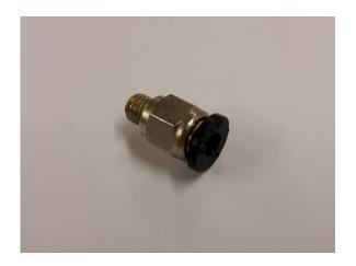
The extruder drive block is printed with an internal thread which matches the thread on the pneumatic fitting. Visually align the fitting with the hole in the drive block, and begin by screwing the fitting in by hand taking car to
