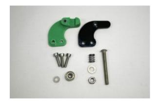
Start by taking the printed lower lever, and insert a M3x12mm cap head screw, as shown.
