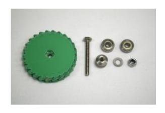
The assembly order for the large gear is M3x25mm hex head screw, Large gear, MR93ZZ bearing, Hobbed insert, MR93ZZ bearing, M3 plain washer, M3 Nylock nut.
